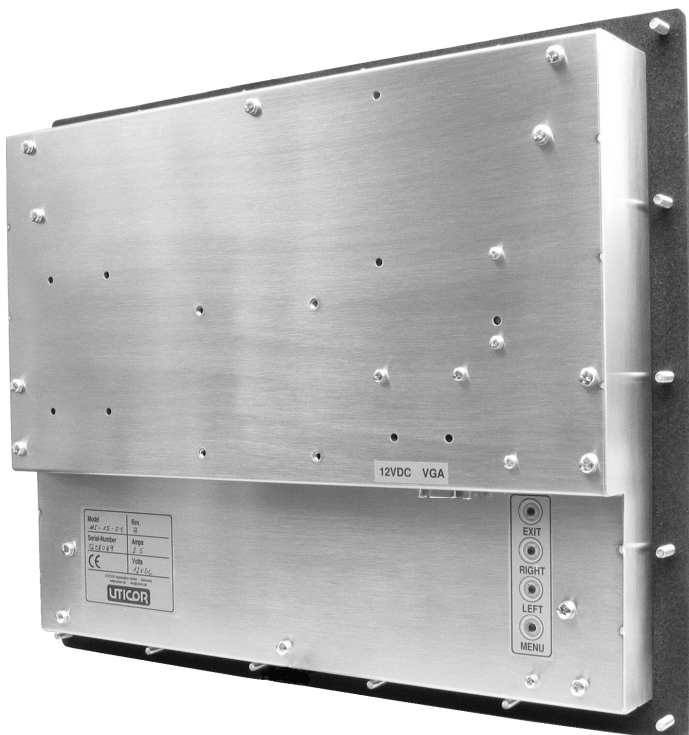
Monitor Back with standard front plate and mounting bolts
